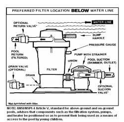
Though the pump is designed for outdoor use, it is strongly advised to protect the electrical components from the weather. Select a well-
