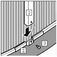
column. The tab must be on the **outside** of the vertical column. Make sure the vertical column is straight up and down.
