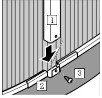
column. The tab must be on the **outside** of the vertical column. Make sure the vertical column is straight up and down.
