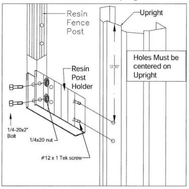
Step 1- Install Post Holders to Pool Upright a-Mark top hole on the pool upright 12½" on center From the top of the Upright, or lower if the top cap support requires. b-Use the post holder to locate the second hole. c-Fasten post holder to upright using two #12 self tapping TEK screws.
