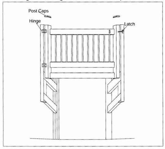
Step 10 Installing latch, hinge, & fence post caps
