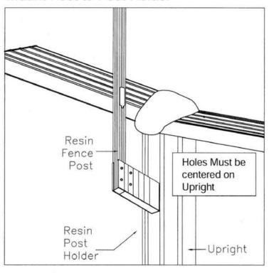
Step 2-Mount Post to Post Holder a-Use two  $\frac{1}{4}$ "-20 x 2" bolts and two  $\frac{1}{4}$ " nuts to mount post to the fence post holder
