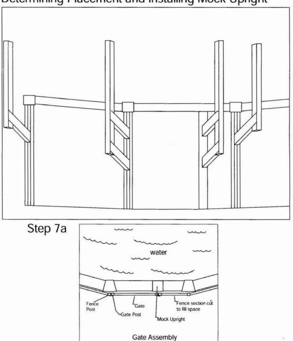
Step 7 Determining placement and installing Mock Upright
