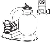
Screw either side of POOL FROG® Cycler on to open nipple end until upright and secure.
