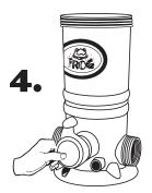
Carefully insert control dial back into housing.
