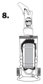
Insert upside down into center of POOL FROG® Mineral Reservoir pushing down firmly on key to puncture seal.
