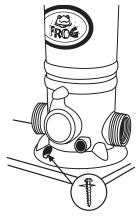
For better stability, POOL FROG® Cycler may be mounted on a base using Phillips pan head screws. One in front and two in back.
