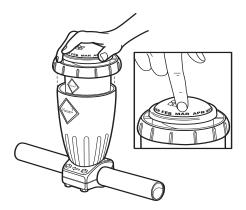
12. Open any valves that you closed and turn on your pool pump to verify that there are no leaks. The small pellets inside the cartridge dome provide evidence of water flow through your Nature<sup>2</sup> Express.
