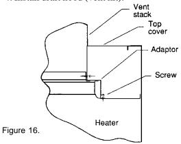
Use provided screws to secure the vent assembly; see Figure 16.
