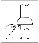
the draft hood; see Figure 15. If the smoke is pulled up into the vent and out of the room, the venting is correct. If it does not, you must make venting corrections.
