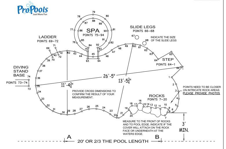
NOTE: MAKE SURE THE A-B LINE IF EXTENDED IS NOT CROSSING THE PERIMETER OF THE POOL.
