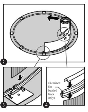
e. Work around the foundation until the entire pool wall is uncoiled into the bottom rails and the top edge is covered with the omega stabilizer and connectors (and beaded liner retainers if you have a beaded pool liner).
