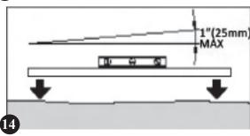
e. **Do not** fill in low areas. Filling will create an unsafe foundation for your pool. Small dips and hollows may be filled in, but the soil must be hardpacked with a tamping tool.
