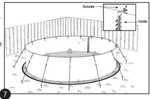
e. Cover the seam and bolt heads on the inside of the pool wall completely with three layers of 2" (50mm) duct tape.
