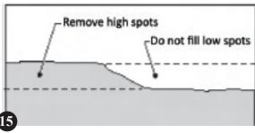
f. Recheck the outer of the circle, where the pool wall will be. Make sure there are no high or low spots. The bottom edge of the pool wall **must** rest flat on the ground and have no gaps under it.
