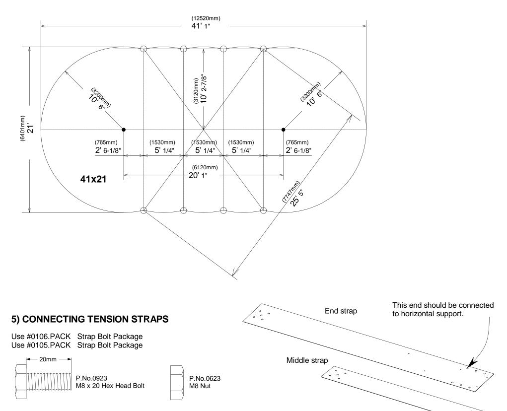
Connect Middle strap(s) to already assembled End straps. Using five sets of M8x20 hex head bolt and M8 nut.
