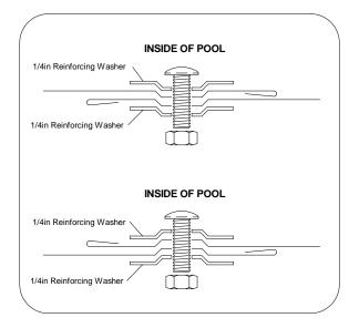
DO NOT FASTEN THE WALL WITHOUT USING THE REINFORCING WASHERS ! FAILURE TO USE REINFORCING WASHERS AS INSTRUCTED WILL CAUSE WALL TO SPLIT WHEN POOL IS FILLED. THIS CAN CAUSE SERIOUS PROPERTY DAMAGE AND/OR BODILY INJURY.
