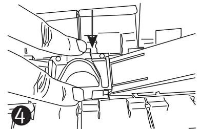
4 Once any debris has been removed or the skirts have been replaced replace the inlet. Note it can only be inserted in one direction and once it is in it should clip on both sides. Note: if it does not clip in then you have it the wrong way around (it is marked L and R).
