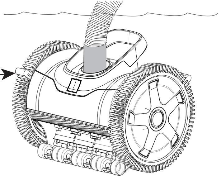
This valve regulates the suction so that the Cleaner does not exceed the optimal 11-14 RPM (revolutions per minute). It does so by opening to bypass water when necessary. This will ensure the best possible performance from your cleaner.
