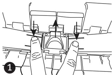
1 Turn the unit upside down and press with both fingers on both sides of the inlet. While pushing down pull up on the inlet.
