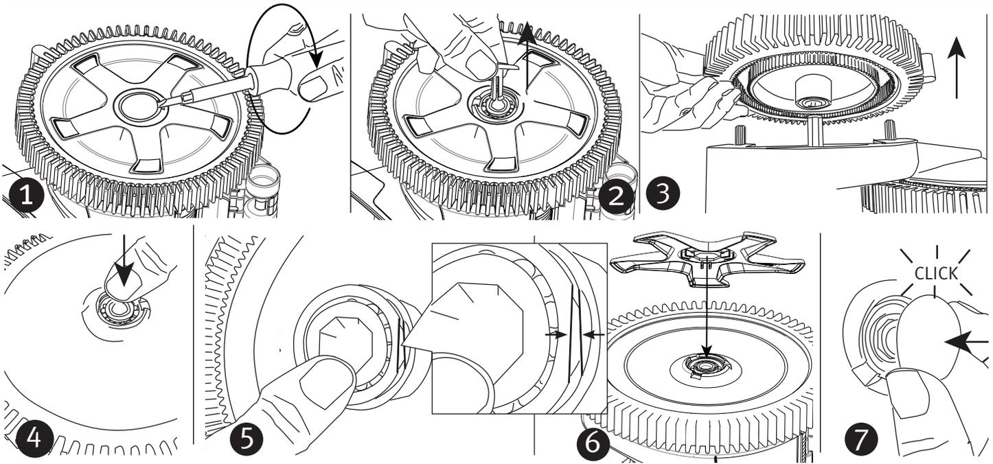
When the unit is reassembled turn the right front wheel (looking from behind) and make sure everything turns smoothly.
