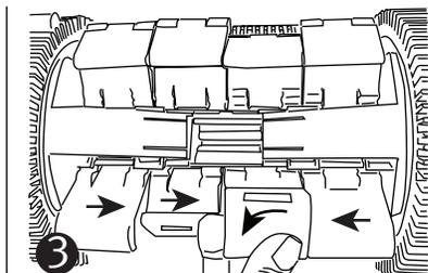
3 Once the inlet is removed you can remove any debris that is in the turbine chamber. You can also remove and replace the skirt/bracket assemblies. One of the middle skirt/brackets can be easily pulled out. Once one assembly is out you can slide the others out easily to replace.
