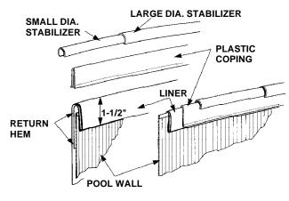
Make a return hem as illustrated. DO NOT cut off excess liner material as the liner will "Slip" from under the plastic coping, causing liner to fall back into the pool. Smooth liner against wall and secure to top of wall with plastic coping. Place stabilizer rails over
