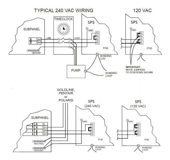
**Note**: Wire the pump directly to the time clock-do not use the CMARSHA as a junction box.
