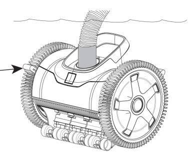
This valve regulates the suction so that the Cleaner does not exceed the optimal 11-14 RPM(revolutions per minute). It does so by opening to bypass water when necessary. This will ensure the best possible performance from your cleaner.
