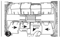
Once the inlet is removed you can remove any debris that is in the turbine chamber. You can also remove and replace the skirt/bracket assemblies. One of the middle skirt/brackets can be easily pulled out. Once one assembly is out you can slide the others out easily to replace.
