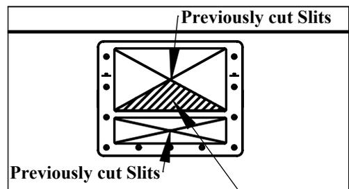
Pull up and out after cutting to remove triangular vinyl from behind horizontal bar.
