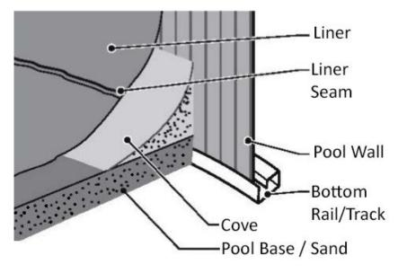
Note: Not all liners are made so the seam is lays on the center of the cove but the seam should run consistently around the pool and be equidistant from the pool wall. The seam
