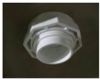
To install the return fitting, you need to un-thread the retaining nut from the fitting. Insert the threads through the pre-punched hole from the inside of the pool and tighten the retaining nut to the back of the fitting. **Be careful not over tighten this nut.**
