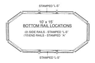
Place bottom rails stamped "L-S" between the side verticals. Place bottom rails stamped "A" on the ends of the pool.
