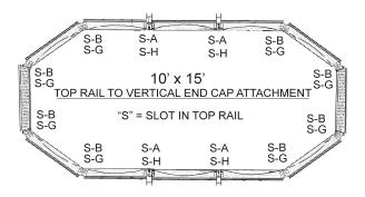
Attach the top rails to the vertical end cap using the hole patterns shown above using #10 x 1/2" screws. Example: On the ends of the pool, attach top rail hole "SLOT" to vertical cap hole "B" and top rail hole "SLOT" to vertical cap hole "G".
