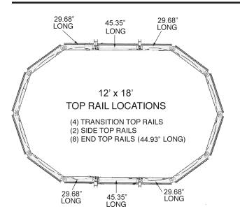
Refer to the diagram above for proper top rail placement.
