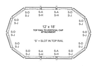
Attach the top rails to the vertical end cap using the hole patterns shown above using #10 x 1/2" screws. Example: On the ends of the pool, attach top rail hole "SLOT" to vertical cap hole "D" and top rail hole "SLOT" to vertical cap hole "J".
