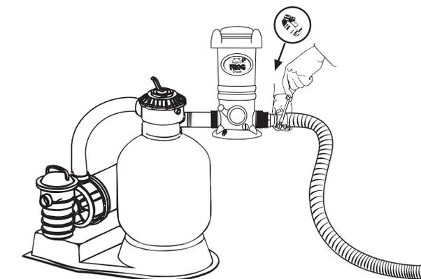
**6.** Attach return section of hose to the adapter with clamp. Tighten clamp with screwdriver.
