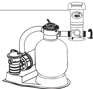
**4.** Apply pipe thread tape or sealant to threaded end of hose adapter.
