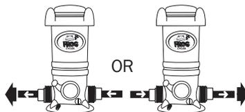
Bi-flow valve design allows installation in either flow direction.
