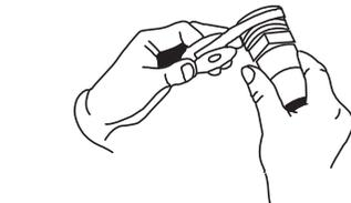
**1.** Apply pipe thread tape or sealant to the threaded end of both hose adapters.
