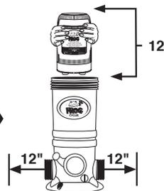
Allow a minimum of 12" above and on each side of POOL FROG Cyclers to ensure room for easy replacement of POOL FROG Mineral Reservoir and Pool FROG Bac Pac.
