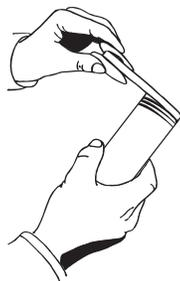
**2.** Screw one end of nipple into the filter return. Hand tighten. Finish tightening by turning 1 to 2 revolutions with a pipe wrench. **DO NOT OVER TIGHTEN.**
