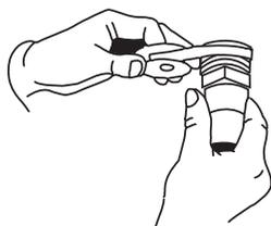
**5.** Screw adapter into the other side of POOL FROG Cyclers. Hand tighten. Finish tightening by turning 1 to 2 revolutions with a pipe wrench. **DO NOT OVER TIGHTEN.**
