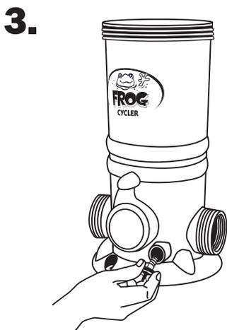
3. Unscrew knob from the front of POOL FROG Cycler. Allow all water to drain.
