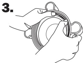
Place your thumbs on each side of the cap over the O-ring in the groove.
