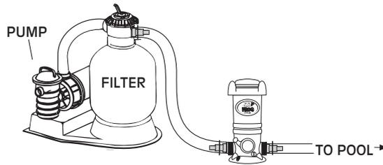
The POOL FROG Cyclor should always be installed between the filter and pool (or between heater and pool if applicable). Never install POOL FROG Cyclor before the heater or damage to the heater could occur.
