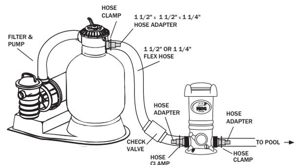
**5.** For better stability, POOL FROG Cyclor may be mounted on a treated wood base using **Phillips pan head screws**, one in front and two in back. If you have questions about stability, please contact your dealer or King Technology.
