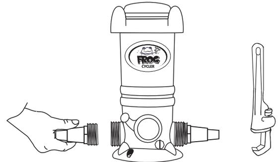
**2.** Screw adapters into each end of POOL FROG Cyclor. Hand tighten. Finish tightening by turning 1 to 2 revolutions with a pipe wrench. **DO NOT OVER TIGHTEN.**
