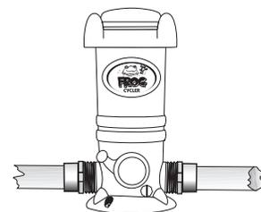
5. Final schematic diagram showing the POOL FROG Cyclers installed in the pool line between the filter and heater, with a check valve installed before them.
