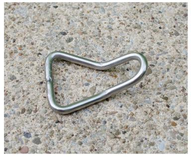
STRAP HOLD DOWN COLLAR -- Designed for elevated spa and deck applications, this collar is used to divert the strap from a vertical orientation to a horizontal direction. This diversion eliminates the need for longer tails that angle down to the main deck level, reducing tripping hazards.
