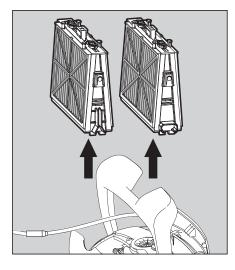
**9.1.1** Open the filter covers and remove the cartridges from both sides of the robot.
