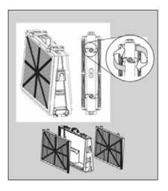
9.1.2 Open the clips and remove the filters.
