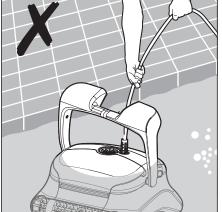
7.4.3 Place the Pool Cleaner on the edge of the pool to let the water drain out.
