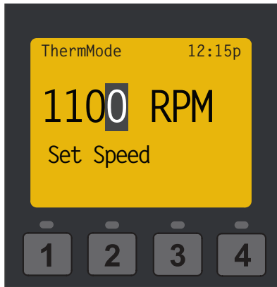
Setting the Thermal Mode Pump Speed
