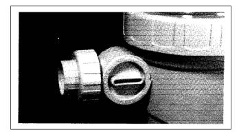
Rotate valve knob counter-clockwise until it stops (open position) for normal pumping operation.
