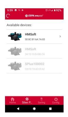
You will be brought to this menu to pair the EVOpool control system (attached to your sand filter valve) with the pump. To skip this step if you are not using the control system, scroll to the bottom and press cancel.
