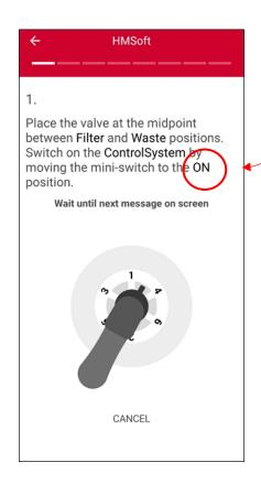
The app will walk you through the steps to calibrate the EVO Pool control system on the sand filter valve handle. The mini-switch is located under cover on the control module. On the last screen, the "Swimming pool features" screen, input you pool volume and answer the 3 questions for a pool heater, salt chlorinator, and pump distance from the pool. This will adjust operation settings and configure the system for your pool.
