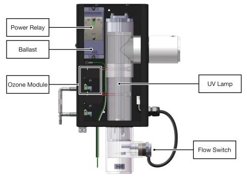
Figure 4: Components (plumbing transparent for clarity)
