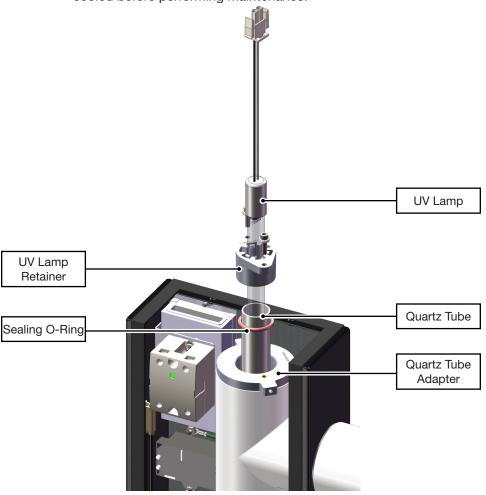
Figure 6: Lamp and Quartz Tube Removal
