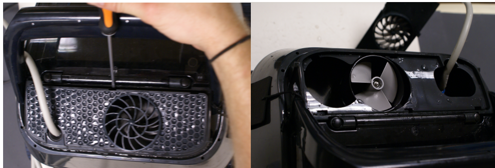
7.1. Use a flat screwdriver to remove the protective grille.
