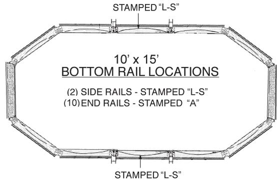
Place bottom rails stamped "L-S" between the side verticals. Place bottom rails stamped "A" on the ends of the pool.
