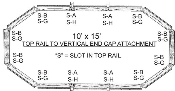
Attach the top rails to the vertical end cap using the hole patterns shown above using #10 x 1/2" screws. Example: On the ends of the pool, attach top rail hole "SLOT" to vertical cap hole "B" and top rail hole "SLOT" to vertical cap hole "G".
