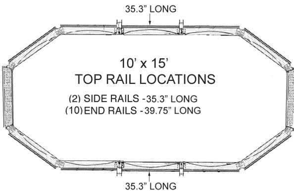
Refer to the diagram above for proper top rail placement.
