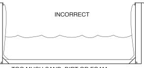
DO NOT ADD MORE THAN 1" - 2" OF SAND, DIRT OR FOAM TO THE POOL BOTTOM, REFERENCED FROM THE BOTTOM OF THE BOTTOM RAIL TOO MUCH SAND, DIRT OR FOAM WILL CAUSE THE LINER TO HAVE WRINKLES
