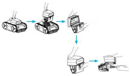
**TIP!** Only spray with a gentle hose, do not use high pressure or basket filter may tear, If filter does not come fully clean use a soft bristle brush to release fixed dirt
