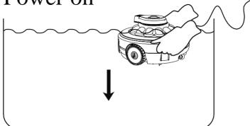
1. Place the cleaner under the surface of the water to allow water to fill it. Loosen the rope attached to the float, place the robot horizontally in the water, turn on the power and wait for the robot to sink freely to the bottom. (A safety feature will not allow the cleaner to operate out of water).
