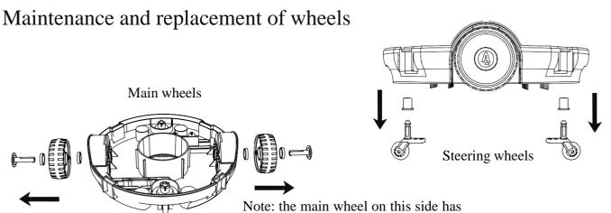
Note: the main wheel on this side has magnets. Contact the supplier for authorized replacement parts. For support and service of your cleaner, please call: +1 888-346-1327
