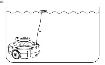
2. Adjust the length of the rope to ensure that the length of the rope is at the same height as the water level, and the extra length of the rope is tied or cut short.
