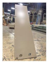
Do not use the two round holes at the base of the buttress support for plumbing runs. These holes are designed to allow the concrete bond beam to flow through for added support. Photo G
