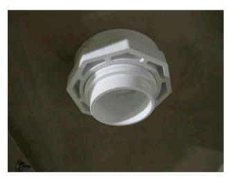
To install the return fitting, you need to un-thread the retaining nut from the fitting. Insert the threads through the pre-punched hole from the inside of the pool and tighten the retaining nut to the back of the fitting. <u>Do not over</u> <u>tighten this nut.</u>
